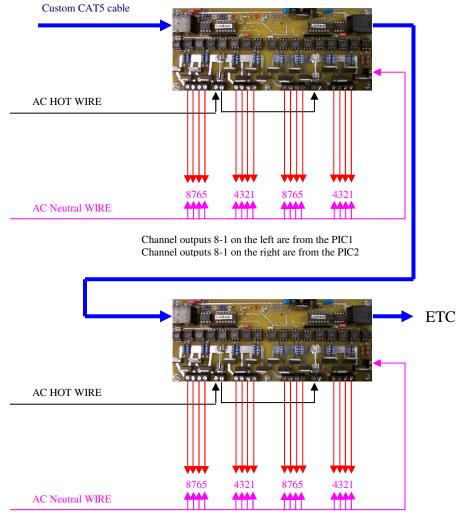
Channel outputs 8-1 on the left are from the PIC3 Channel outputs 8-1 on the right are from the PIC4
