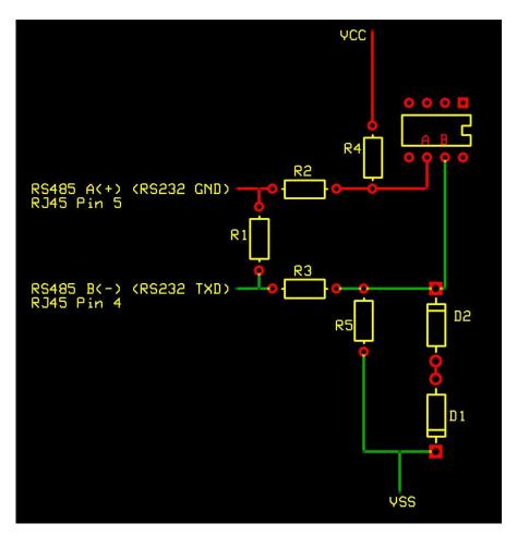
R1 = 120 R2, R3 = 1K R4, R5 = 27K D1 = 1N5229 D2 = 1N5239 U1 = The chip is any RS485 chip.
